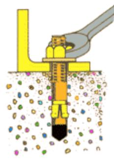
3. Tighten nut until wrench resistance is felt (approximately 3 to 4 turns of the nut after snugged up) anchorage is now complete.
